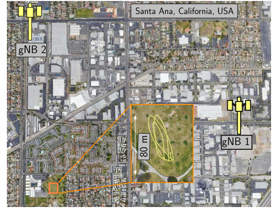
Fig. 9. Environment layout and UAV trajectory for the 5G NR UAV experiment.
