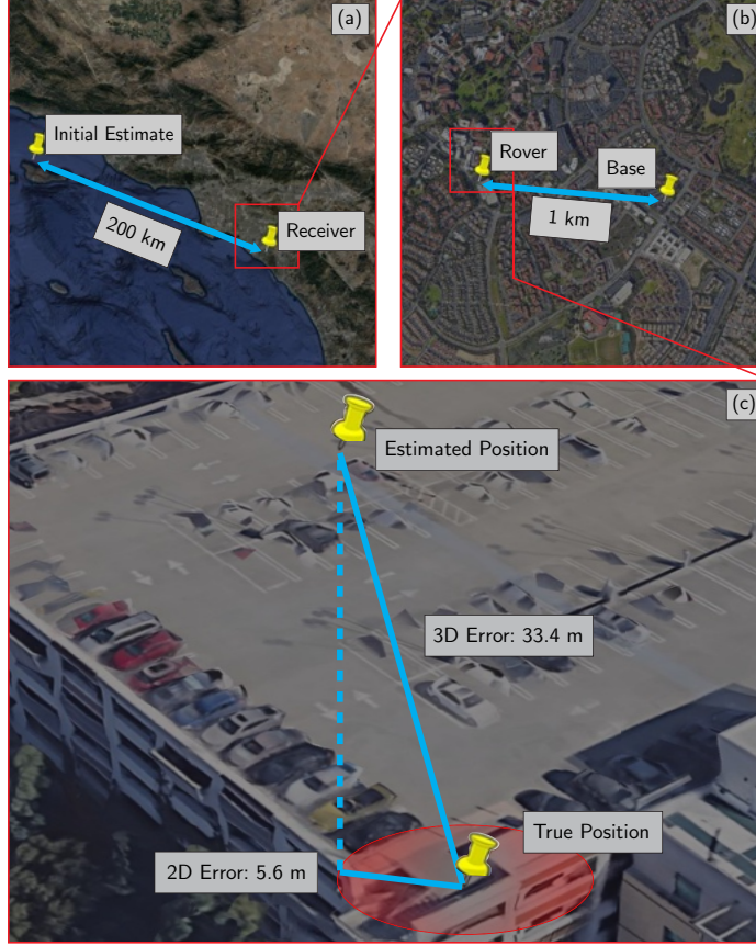
Figure 6.10: (a) Rover's initial position estimate, (b) Base's and rover's position, and (c) Rover's true and estimated position.
