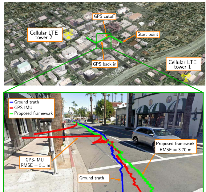
Fig. 18. Environment 2 experimental results: environment layout, LTE SOP tower locations, true vehicle trajectory, and the different navigation solutions, where the estimated vehicle position obtained from GPS-IMU and the proposed method are shown using red and green lines, respectively. In this experiment, the vehicle-mounted receiver traversed 345 m in an urban street while listening to only 2 LTE SOPs simultaneously. Image: Google Earth.
