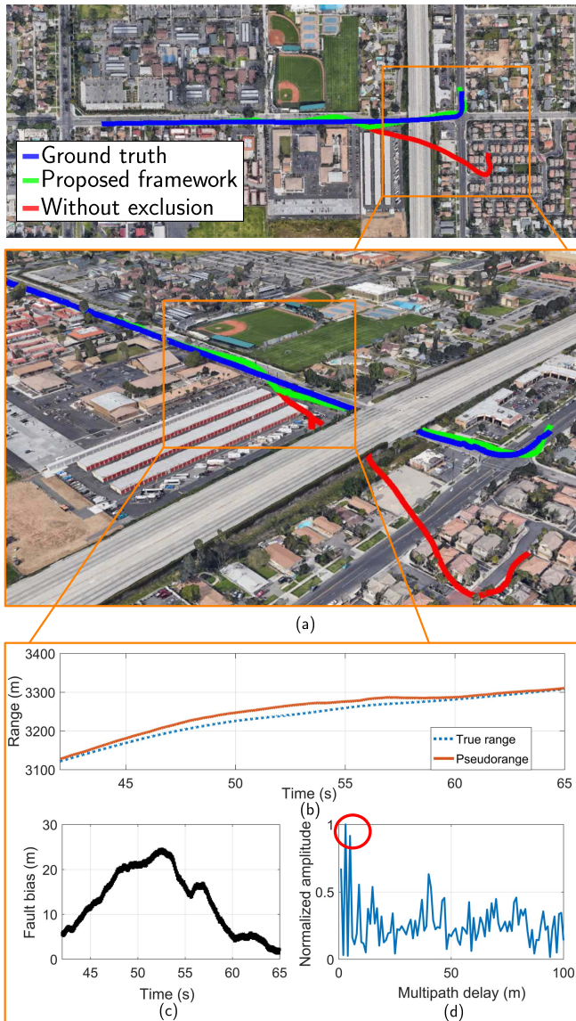
Fig. 17. Environment 1 experimental results: (a) A comparison between the vehicle’s ground truth trajectory versus its estimated trajectories with and without measurement exclusion. As can be seen, the proposed framework outperforms the navigation solution without measurement exclusion. (b) The recorded true range versus pseudorange. (c) The fault bias added to the measurement. (d) Receiver CIR.
