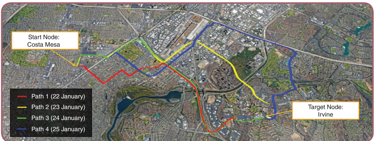
FIG 10 The four candidate paths between Costa Mesa and Irvine. GNSS signals along the paths were collected during four consecutive days.
