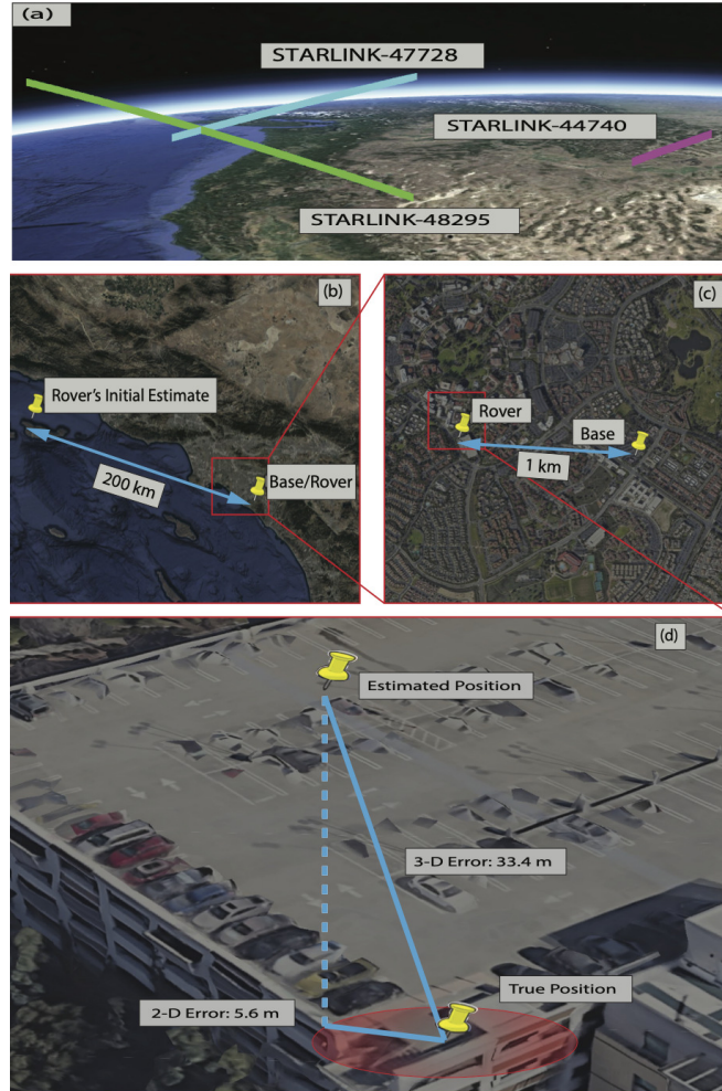
Figure 6: (a) Starlink LEO SV trajectories, (b) rover's initial estimate compared to the base/rover's locations, (c) base and rover locations, and (d) true and estimated rover's positions.
